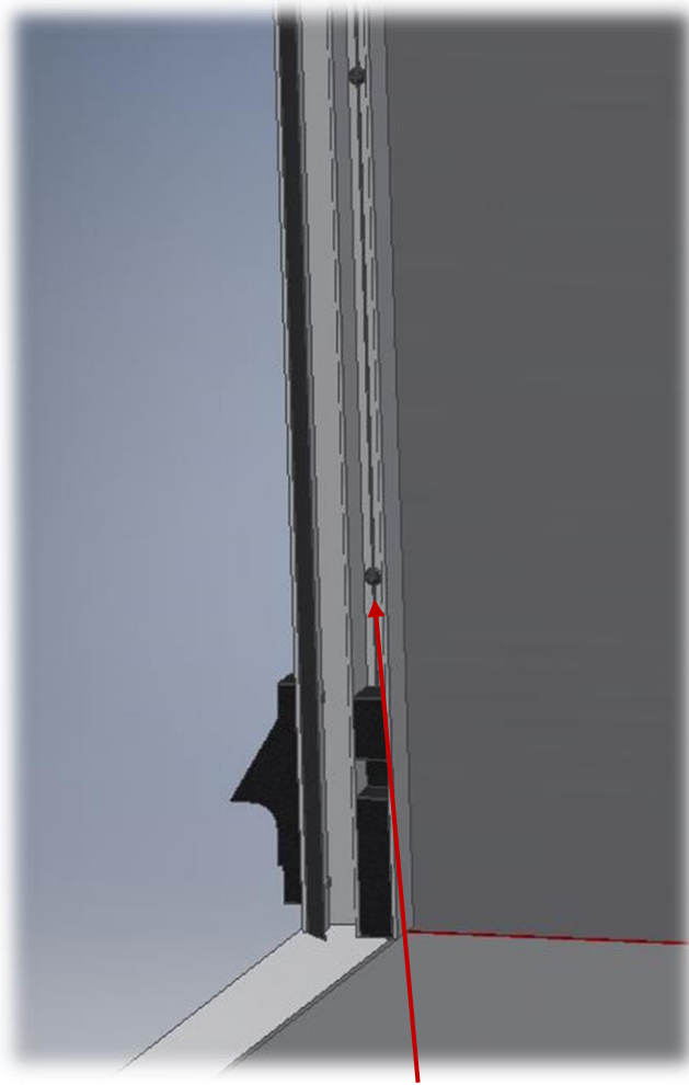
Picture 8 - Fixing E type runner profile
